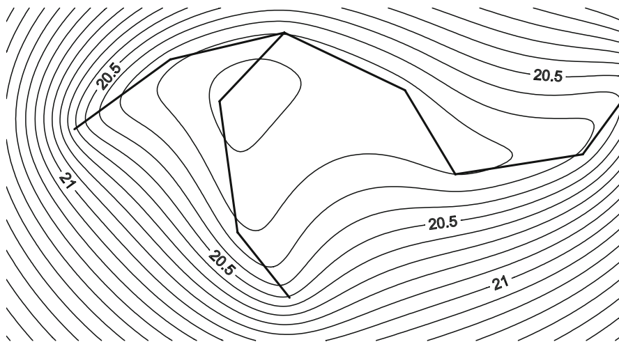
Fig. 11 Piezometric contours in the lower aquifer; note that the elements are not in the lower, but in the upper aquifer. The lowest head is along the shortest closed contour and is 20.1 m
